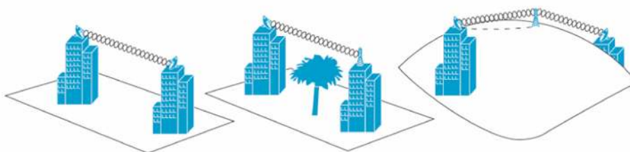
Figure 2. Crossing Great Distances with Cisco Aironet Bridge Antennas
